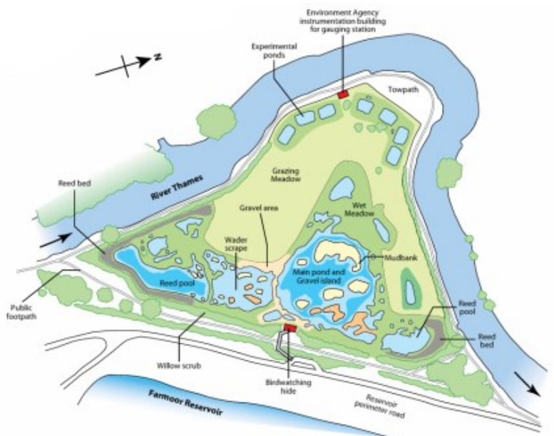
Figure 4 Diagram illustrating the creation of floodplain along the River Thames on Pinkhill Meadow in Oxfordshire (image from RRC Manual of Techniques )
